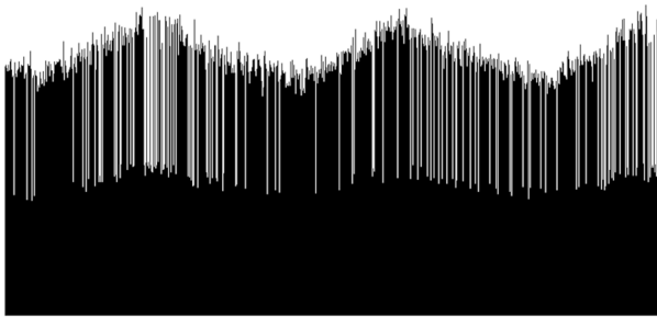
Fig. 5. Total ping energy levels. The horizontal axis denotes the series pings and the vertical axis denotes the average intensity of each ping.
