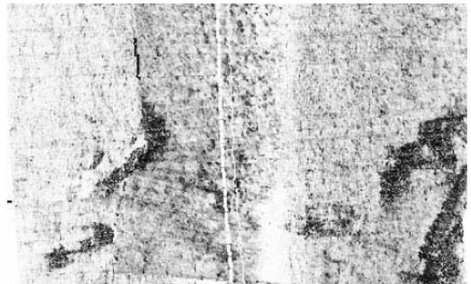
Fig. 11. Mosaic image patched by interpolation algorithm [6]. The most across-track gray lines overlay the images are patched lines.
